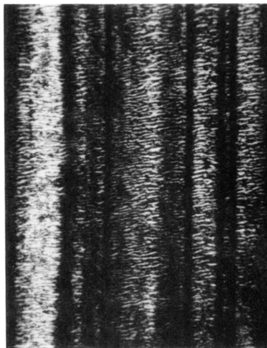
Figure 7. Photomicrograph of a unidirectional smear of poly(chloro-1,4-phenylene trans -hexahydroterephthalate) at 240 \times magnification.
